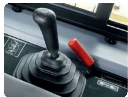
Remote safety lock levers
