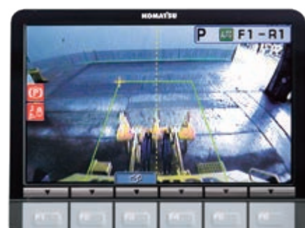
Fully integrated rear-view camera system
