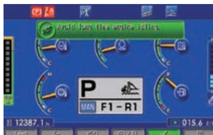
Eco-gauge, Eco guidance and fuel consumption gauge
