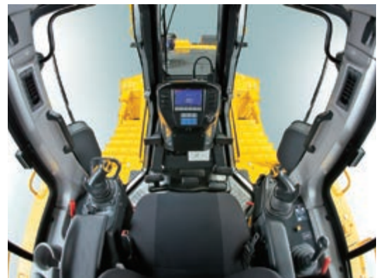
Fully air suspended operator station ensures maximum operator comfort and an excellent view on the blade.
