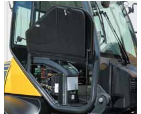
Side cover for quick maintenance access
