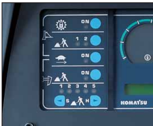
Track shoe slip control panel
