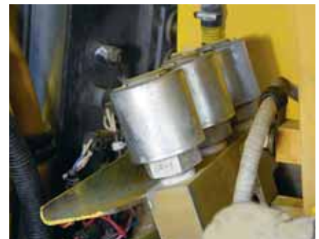
Canister-type breathers facilitate checking and cleaning (optional)
