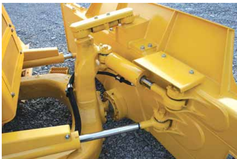
Straight Power Angle Tilt blade with adjustable pitch
