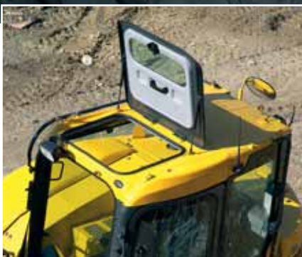
Opening skylight for overhead visibility
