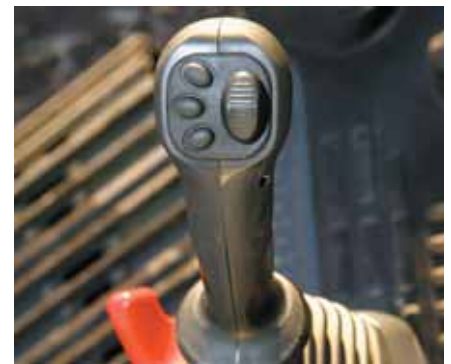
Joysticks with proportional control button for attachments
