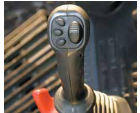
Joysticks with proportional control button for attachments
