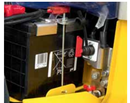
The battery main switch is standard
