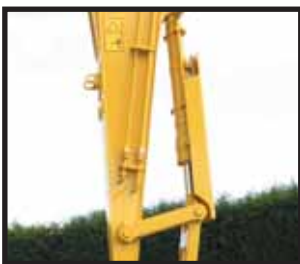
Attachment cylinder guard offers protection against falling objects
