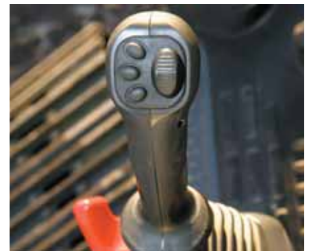
Joysticks with proportional control button for attachments
