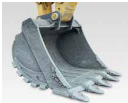
Komatsu bucket with Kmax teeth
