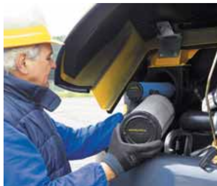
Rear bonnet for quick engine check and access to maintenance points from ground level
