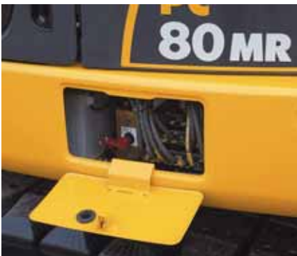
The battery main switch is standard
