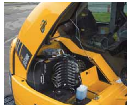
Right bonnet for easy access to main control valve, fuel tank, oil tank and tool box
