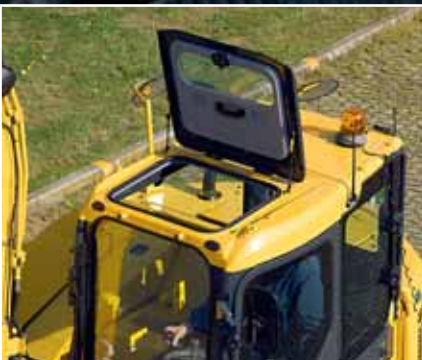
Opening skylight for overhead visibility
