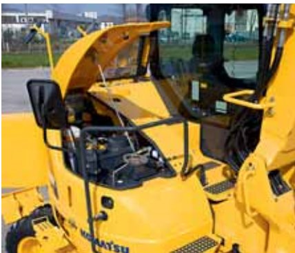
All major maintenance points can be easily reached from ground level
