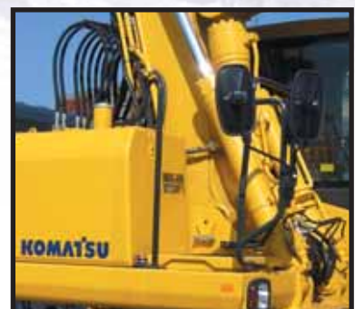
Large handrail for safe access
