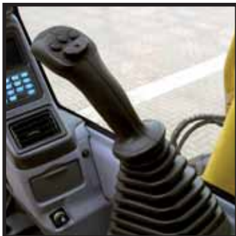
Joysticks with proportional control button for attachments
