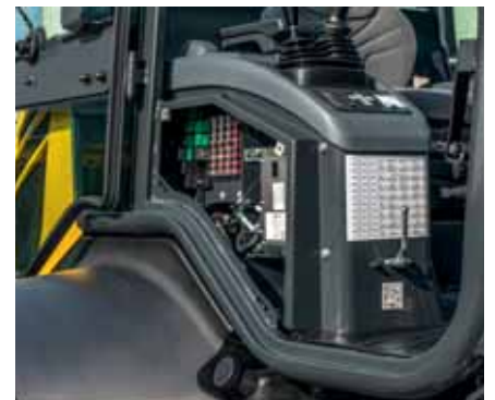
Side cover for quick maintenance access
