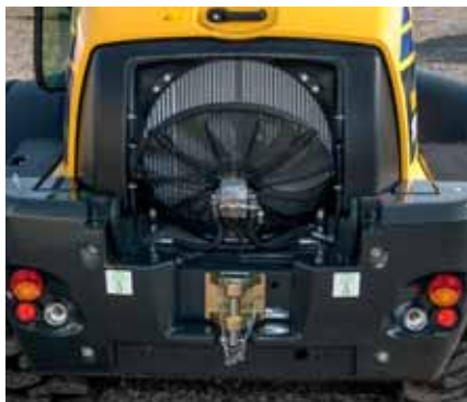
Tiltable radiator fan for convenient cleaning access
