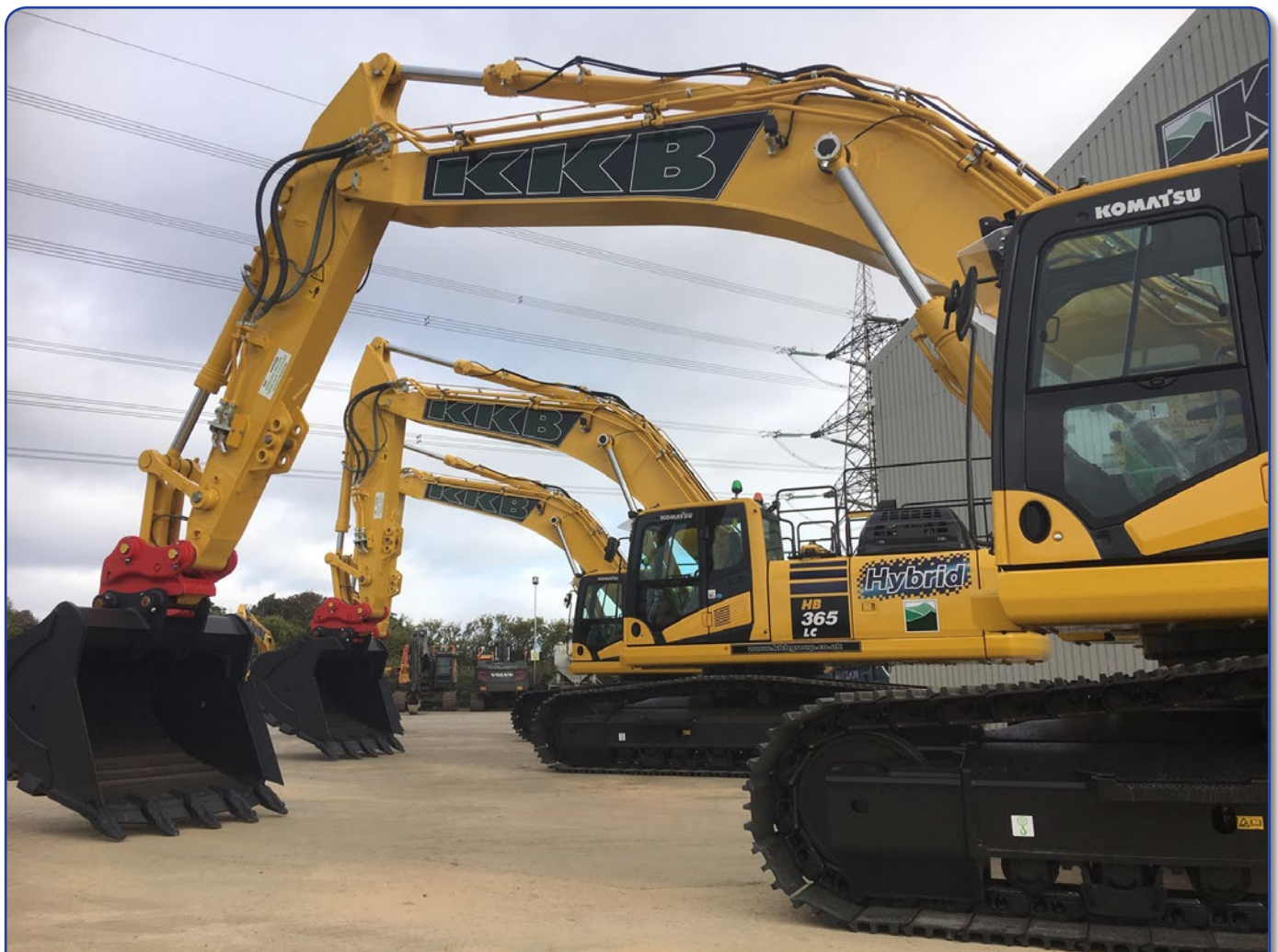
Tasks involving lots of slewing are where the Komatsu Hybrid system can deliver significant savings.
