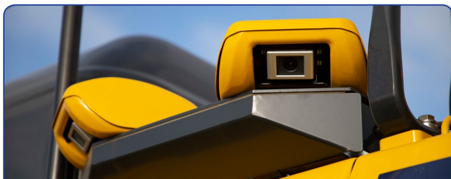
Komatsu KomVision™ camera system is standard on the HB215LC-3.
