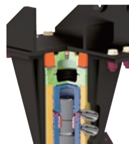
Nitrogen accumulator Constant power over time
