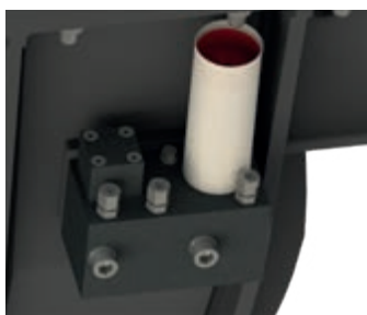
Automatic greasing system Optional on JMHB100H-1, standard on all larger models
