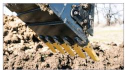
Marubeni Komatsu was able to retro-fit the bucket with Kprime Teeth new heel and vertical shrouds
