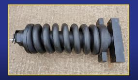
Adjustments are made by pumping or draining grease through the track adjuster valve. Incorrect adjustment will seriously impact the lifetime of the undercarriage.
