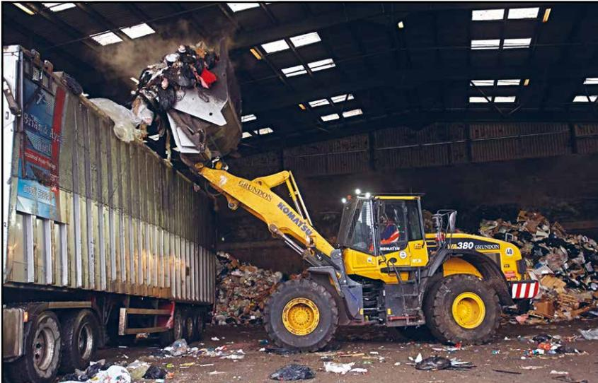
**“Super Highlift” loader arms and Toe-tip bucket enable the Komatsu to load the highest trailers in complete safety.**
