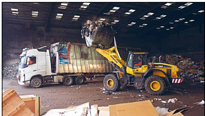
With a full bucket and a steady hand, operator Nigel Eaton sets to loading an articulated refuse bulker. The WA380-7 has full "Waste Handler" package.
