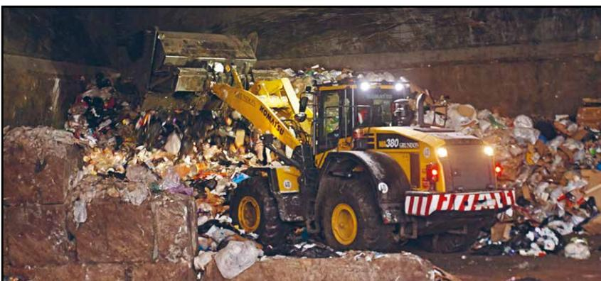
**Get in there! Here the Komatsu is used to trim the pile and make room for the next RCV on the tipping floor.**
