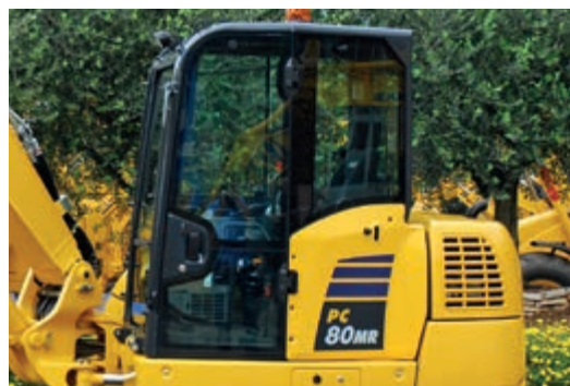
Newly designed cab, with control elements from larger machines. Features such as standard air condition and a hinged door ensure maximum operator comfort.
