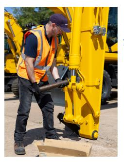
Pins & bushes may seem like minor components, but they play a vital role in the smooth & precise operation of your excavator. If pins & bushes are not changed over time, work quality can suffer:
