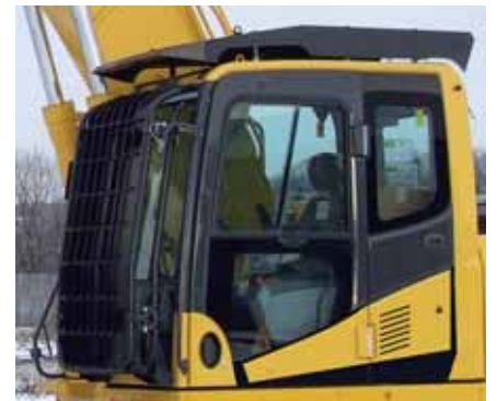
Falling Object Protection System (FOPS) optional
