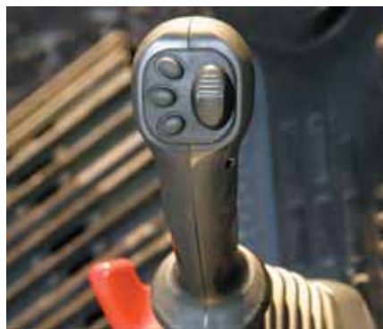
Joysticks with proportional control button for attachments
