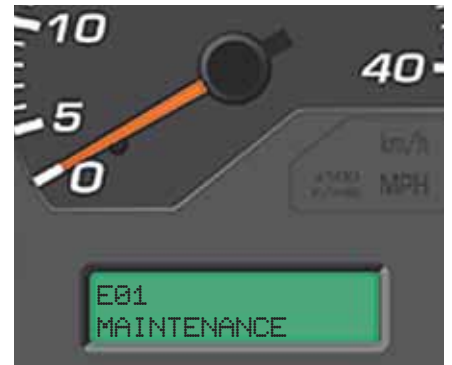
EMMS (Equipment Management Monitoring System)
