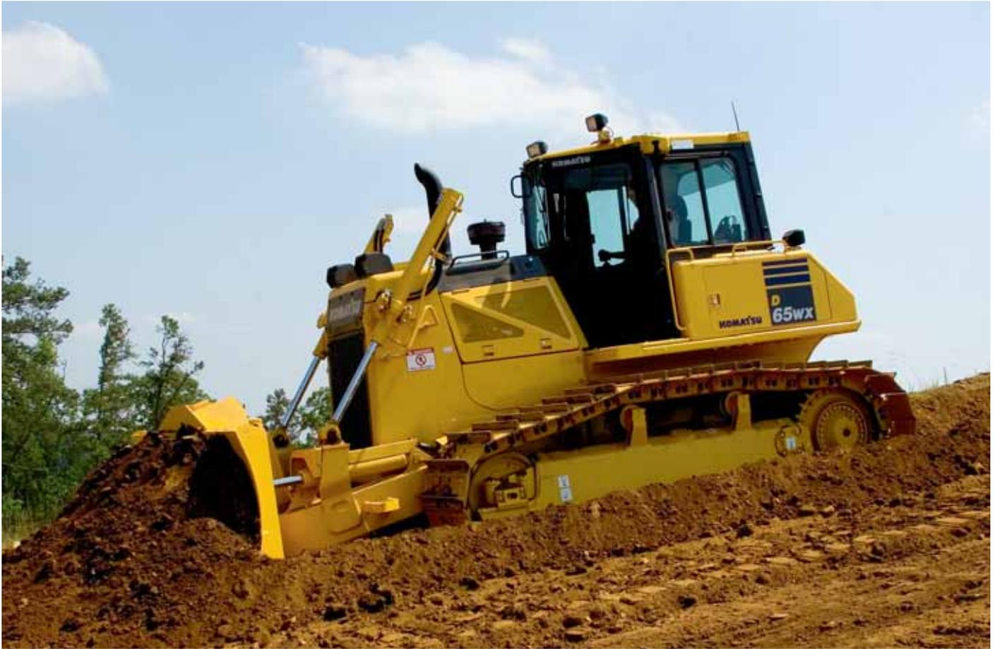
The HD-AIR Track was developed by Komatsu for D65 bulldozers. It features AIR bushings that are more impact resistant than on the standard track and more flexible than on the AR track, making the track suitable for both abrasive and impact applications. It is also equipped with Heavy Duty links that are bigger and more durable than standard ones.
