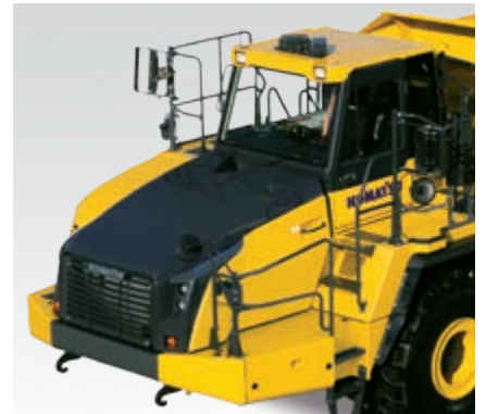
Built-in ROPS/FOPS to ISO 3471 and SAE J1040-1988c standards
