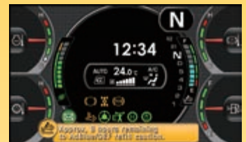
AdBlue® level and refill guidance
