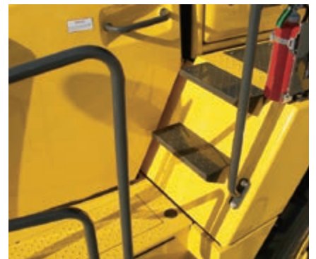
Safe cab access with handrail, away from the potentially hazardous articulation
