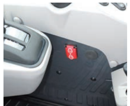
Secondary engine shutdown switch
