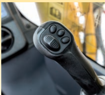
Joysticks with proportional control button for attachments.
