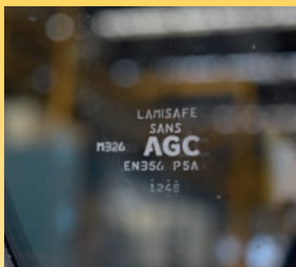
High impact protective glass (compliant with EN356 grade P5A) is fitted to front and roof window. Roof window wash/wipe system is fitted as standard.
