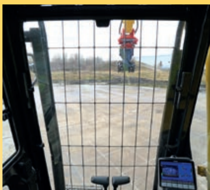
Carefully aligned grid layout ensures maximum visibility with correct protection. One piece front screen fitted with high impact protective glass.
