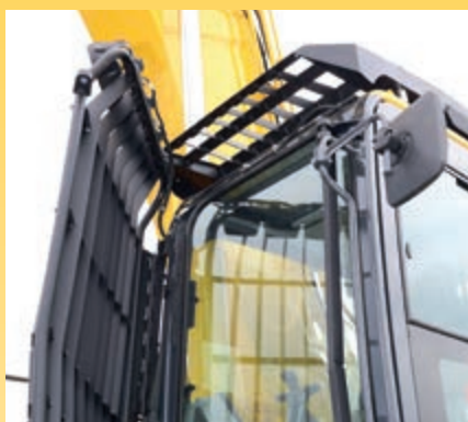
Hinged front guard to allow easy access for windscreen cleaning. The Demolition Safety SpaceCab™ is ROPS compliant with ISO 12117-2:2008.
