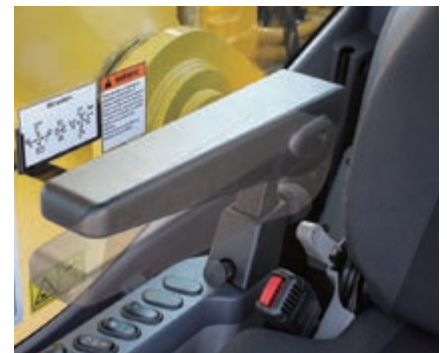
Armrest with simple height adjustment
