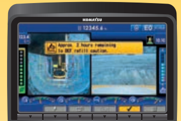
AdBlue® level and refill guidance
