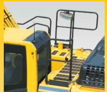
Hand rails and anti-slip plates
