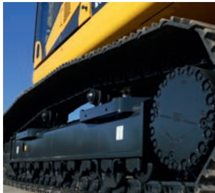
Full length track roller guards (optional)
