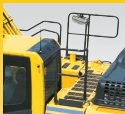
Hand rails and anti-slip plates
