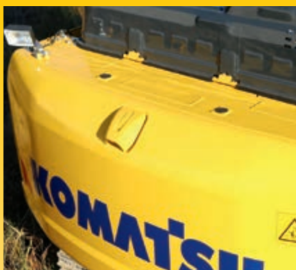
Rear-view and optional side-view camera
