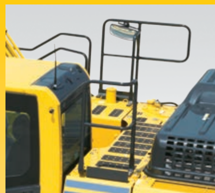
Hand rails and anti-slip plates
