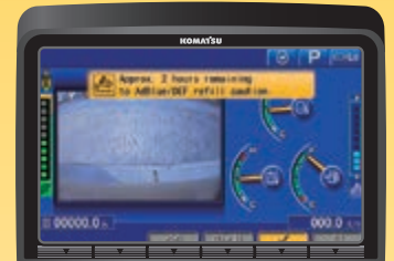
AdBlue® level and refill guidance
