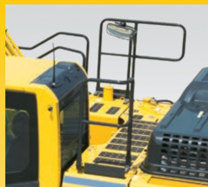
Hand rails and anti-slip plates
