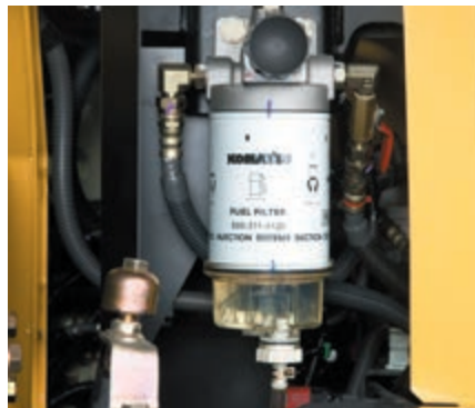
Fuel pre-filter with water separator
