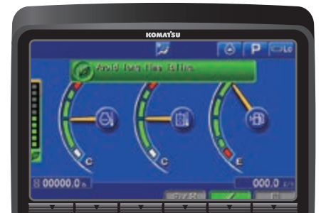
Eco-gauge, Eco guidance, idle caution and an adjustable idle shutdown all contribute to further reduce fuel consumption
