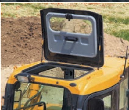
Overhead visibility and opening skylight
