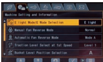
New E-Light engine mode enables increased fuel savings compared to current Economy mode
