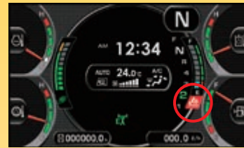
AdBlue® level gauge and refill guidance
