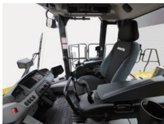
New operator seat with integrated EPC lever console and optional joystick steering
