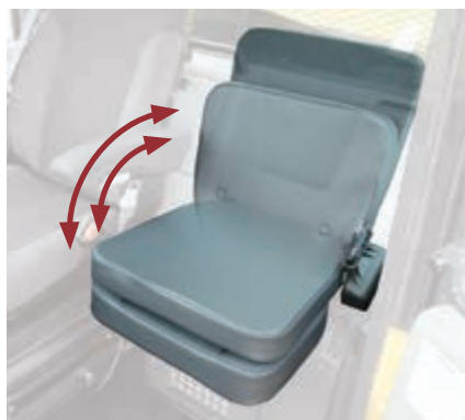
The full size trainer seat has a foldable cushion and back rest for easy cab entry and access to the air conditioner filter and glove compartment
