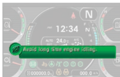
Eco guidance supports energy saving in real time (e.g. avoid long time engine idling)
