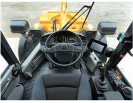
New operator seat and optional new joystick steering for maximum operator comfort.
