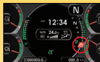
AdBlue® level gauge and refill guidance
