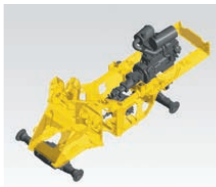
Robust torsion-resistant main frame
