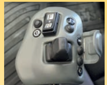
Komatsu short lever steering (K-SLS) (option)
