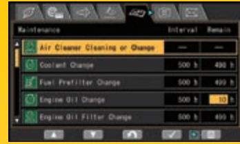
Basic maintenance screen
