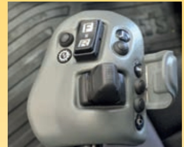
Komatsu short lever steering (K-SLS) (option)
