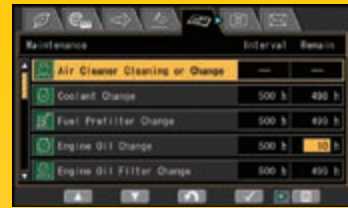
Basic maintenance screen
