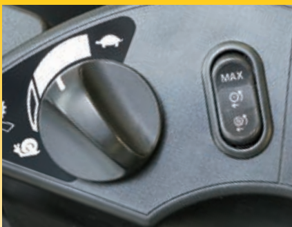
Variable shift control dial with new creeping speed range (left) and variable traction control system switch (right)
