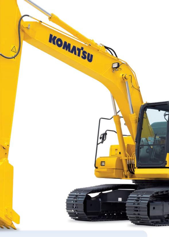
Engine power 90 kW / 121 HP @ 2100 rpm Operating weight **18180 - 18885 kg**  Bucket capacity max. 0.94 m<sup>3</sup>
