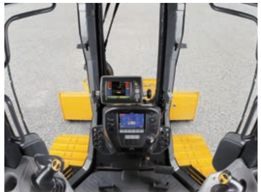
Maximum operator comfort and an excellent view on the blade due to the super-slant nose design.
