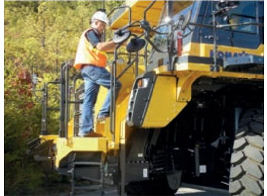
*Safe and convenient cab access thanks to stairway with handrail*
