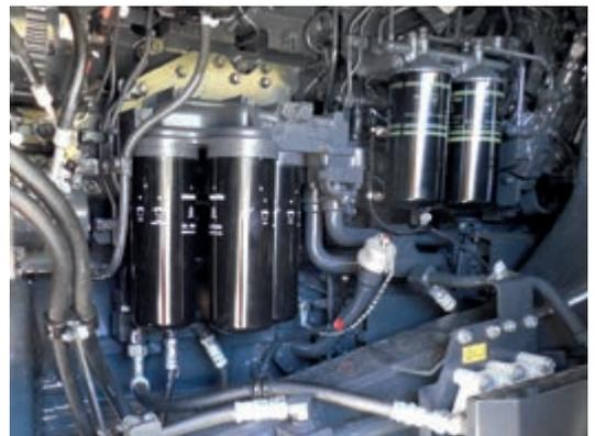
*Centralized greasing points and filter arrangements make maintenance easier*
