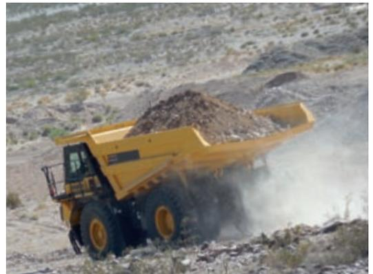
*Auto Retard Speed Control (ARSC) allows the operator to simply set the downhill travel speed and go down slopes at a constant speed.*
