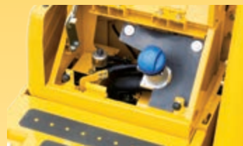
For simple access, the AdBlue® tank is installed on the front stairway
