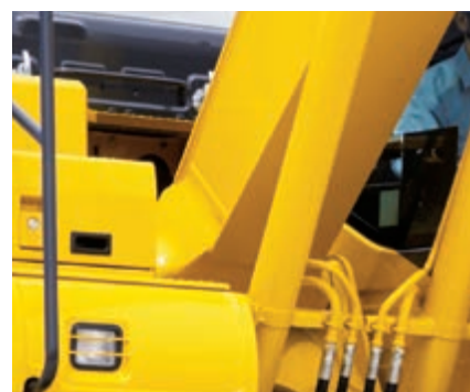
Cast boom foot and single piece boom plates
