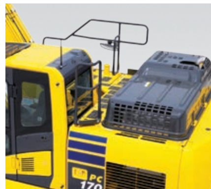
Hand rails and anti-slip plates
